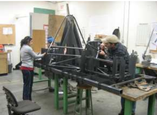
Fitting chassis tubes in the jig
