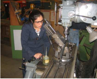
Milling the chassis tubes
