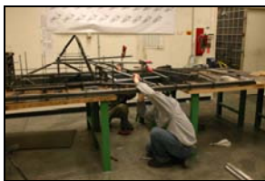
Test Fitting Tubes
