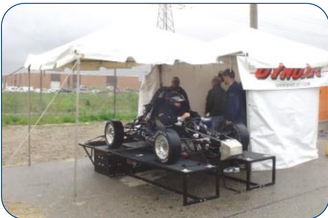
ABOVE LEFT: Dynamometer testing at the competition
