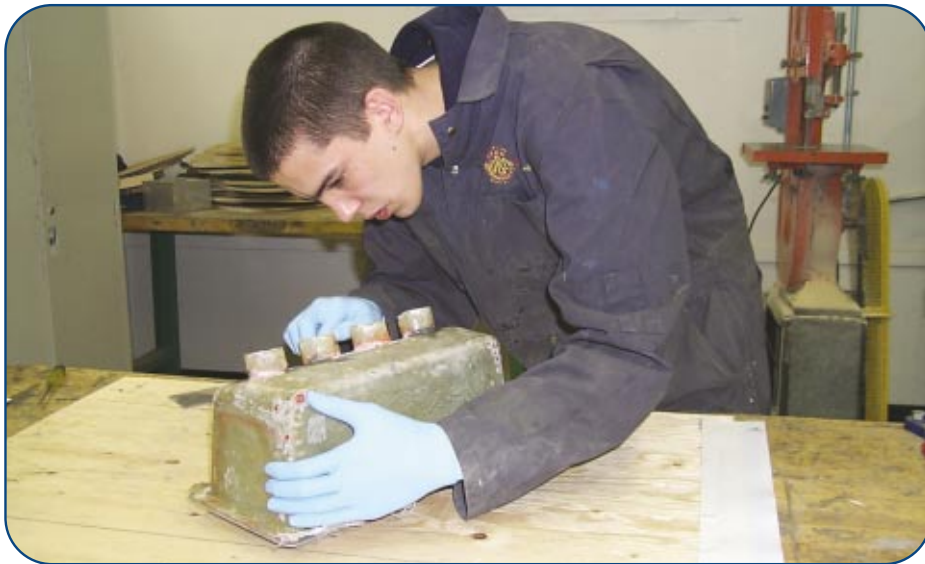
BELOW: Eric Kastanis laying fibreglass over the air box mould.
