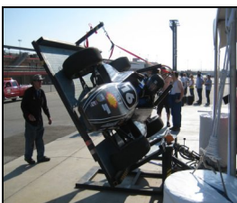
Tilt Table Leak Test
